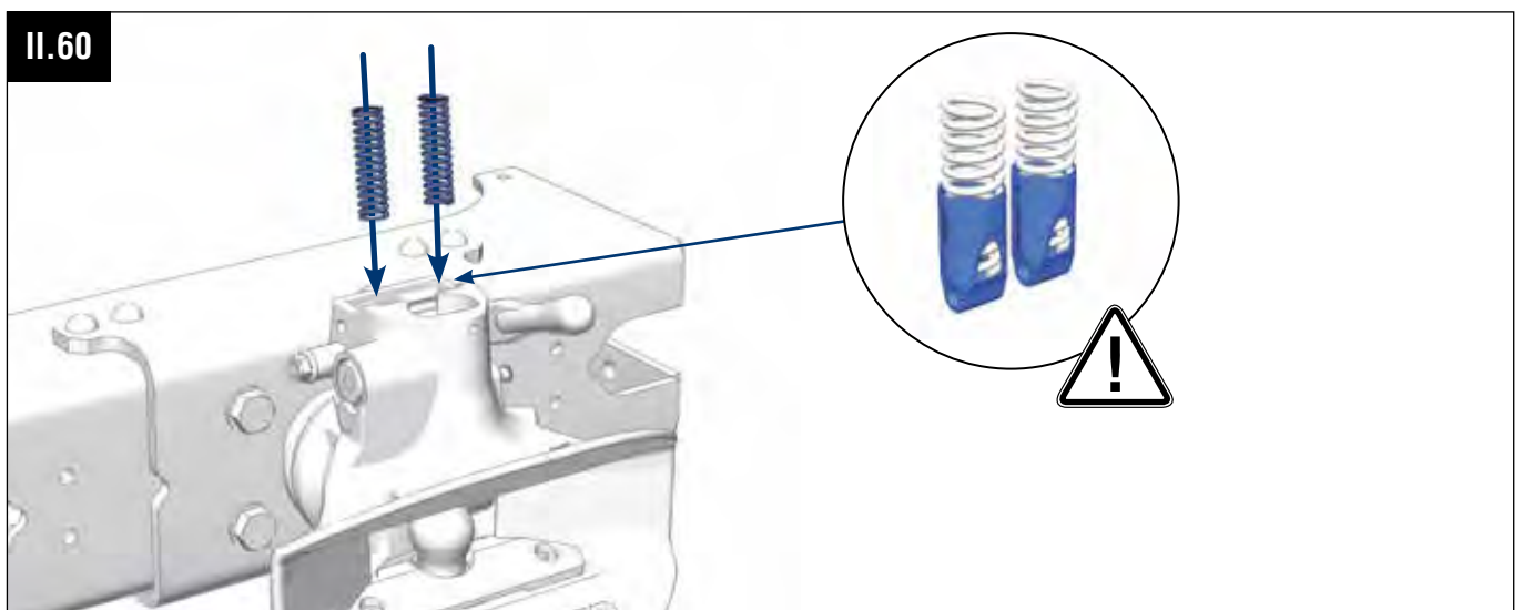
Montage Schließfedern Fitting of closing springs
