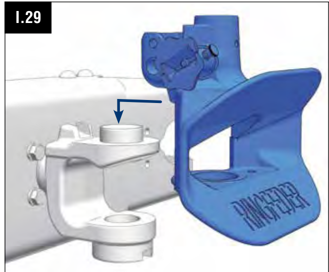
I.29 Montage des Kuppelkörpers Fitting of the coupling assembly
