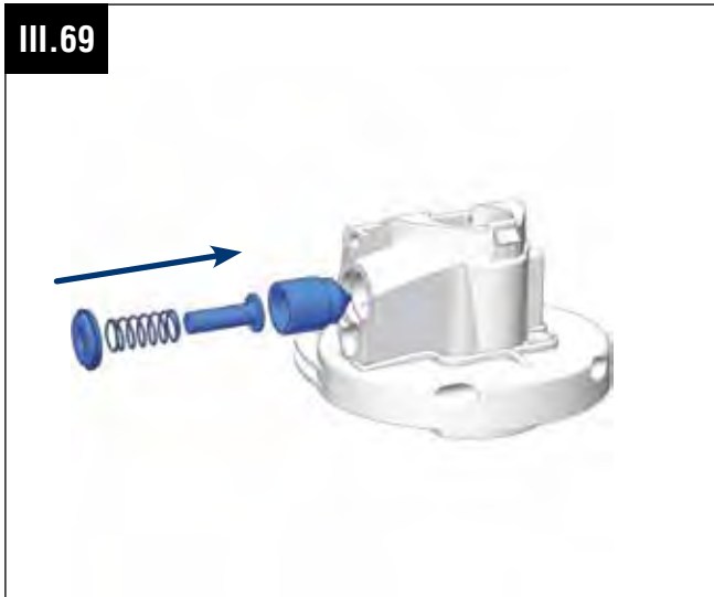
Montage Sicherung (1) Fitting of safety device (1)
