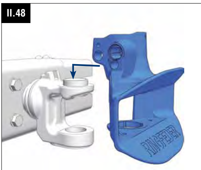
Montage des Kuppelkörpers Fitting of the coupling assembly
